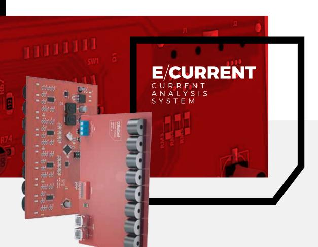
E/Current is especially designed to capture current graphs of railway switch point systems which can also be used current measurement of switch heating system.
